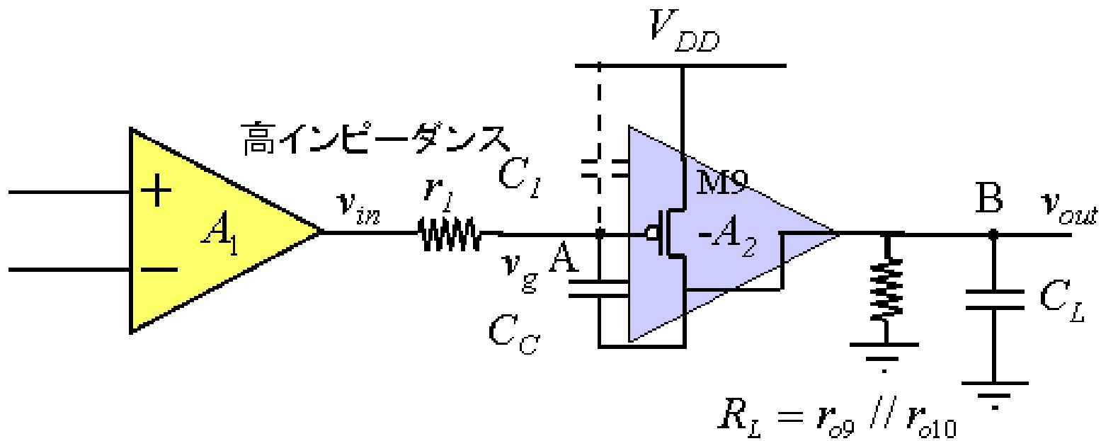
$$A_V(s) \equiv \frac{v_{out}}{v_{in}} \approx \frac{R_L(g_{m9} - sC_C)}{s^2 R_L r_i (C_L C_C + C_L C_1 + C_C C_1) + s R_L r_i g_{m9} C_C + 1}$$
