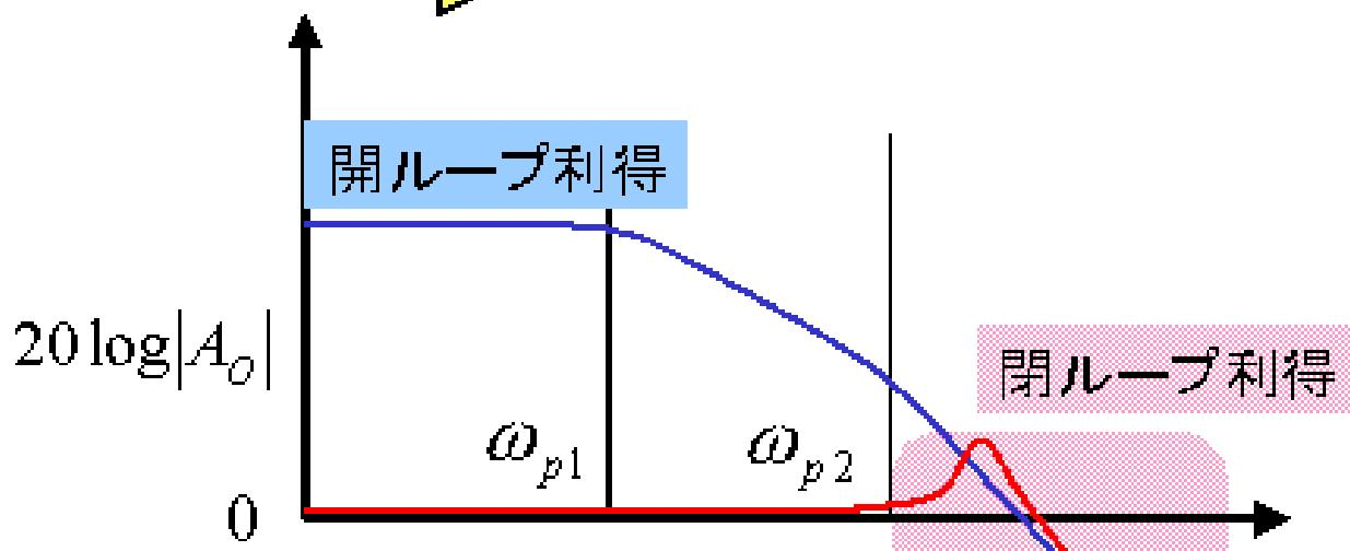
$$A(s) = \frac{A_o}{(I + \frac{s}{\omega_{p1}})(I + \frac{s}{\omega_{p2}})} \xrightarrow{\text{ブロック線図}} A_C(\omega) = \frac{A_o}{I + A_o} \approx \frac{1}{I + j \frac{\omega}{A_o \omega_{p1}} + j^2 \frac{\omega^2}{A_o \omega_{p1} \omega_{p2}}}$$
