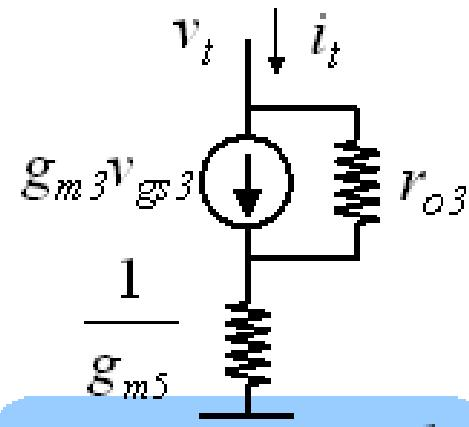
$$\frac{v_{gs9}}{v_{II}} = \frac{R_3}{\frac{1}{g_{m1}} + R_3} \cdot \frac{\frac{1}{g_{m5}}}{R_3} = \frac{\frac{g_{m1}}{g_{m5}}}{1 + \frac{g_{m1}}{g_{m3}}}$$
