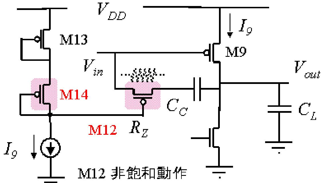
$$R_Z = \frac{1}{\beta_{12}(V_{GS12} - V_{Tp})} = \frac{\beta_{14}}{\beta_{12}} \cdot \frac{1}{g_{m14}}$$
