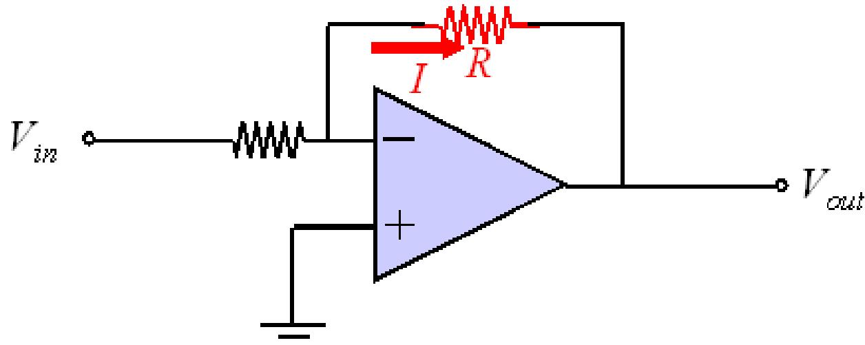
$$V_{out} = IR = IR_0(1 + \alpha\Delta T) = IR_0(1 + \alpha\beta I^2 R)$$
